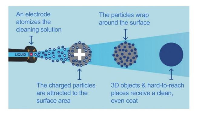
Electrostatic technology helps reduce the material consumption and improve the surface coverage, thus increasing the spraying efficiency enormously.
